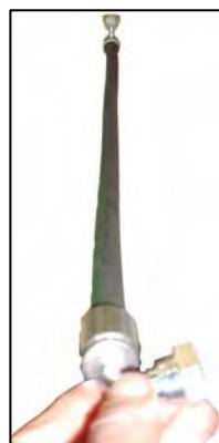
*Keep straight the further end and rotate clockwise the closest end of the requested angle.*
