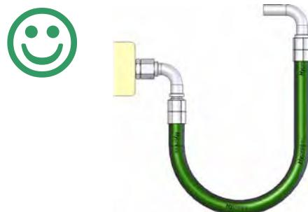
Too tight bend may kink the hose, restrict or stop the fluid flow, or damage the hose reinforcement.
